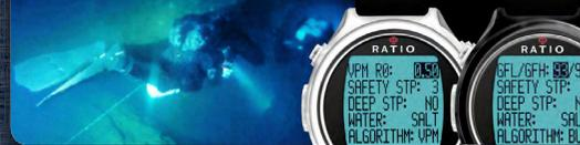
User settable **last Deco Stop depth**, User settable **Safety Stop**, and **Deep Stop**.
